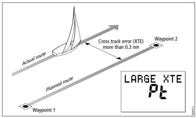
Cross track error (XTE) is the distance between the current position and a planned route. The SmartPilot receives the cross track error information
